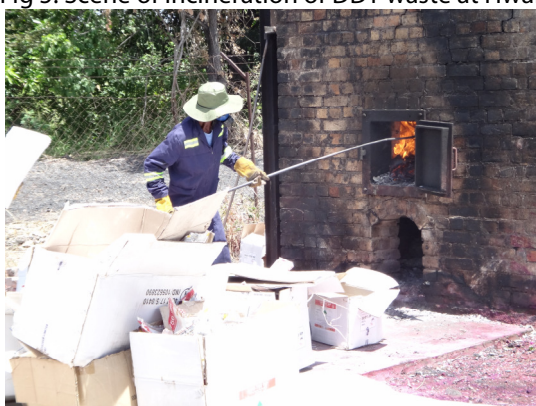
Fig 5: Scene of incineration of DDT waste at Hwange Colliery, Mat. South Province
